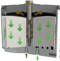
By removing up to 99.9% water contamination. the production of acids (hydrolysis) is inhibited. As the oil passes through the element, minute particles of carbon, wear metals and silicon are extracted from the oil by adhering to the many surfaces of the filter.
